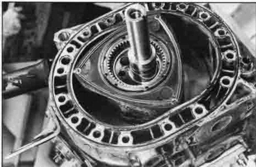
Inside the futuristic Wankel chambers: light carbon deposits and normal seal wear
