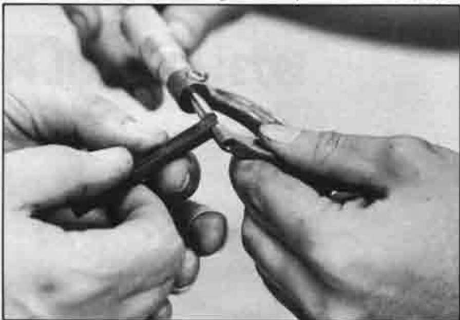
An aluminum-impregnated carbon apex seal under micrometer scrutiny
